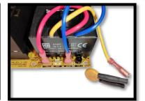
**Step 3.** Disconnect the BLUE cable spade connector from the "BLUE" spade and re-connect it to the free spade of the varistor assembly supplied in this pack.
