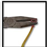
**Step 2.** Disconnect the RED cable spade connector from the "240V" spade and re-connect it to the spade marked "NC".
